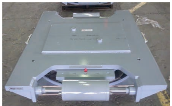
TP integrated with shock absorber (TSTD) and hysteretic steel device (TEPD)
