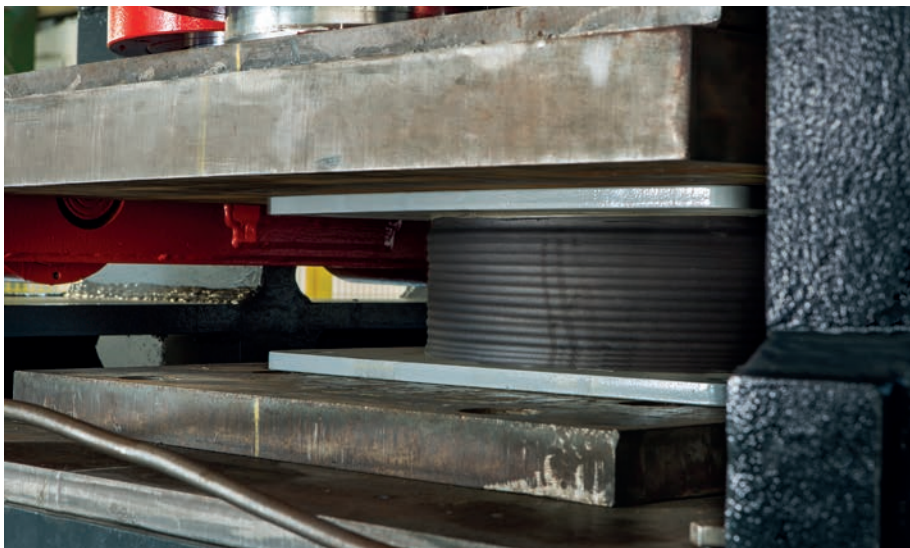
Horizontal stiffness test on rubber bearing
